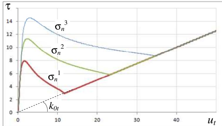
Shear stress versus slip under different compressive normal stresses for the option without plasticity: the curves join and follow the elastic line with residual stiffness  $k_{0t}$
