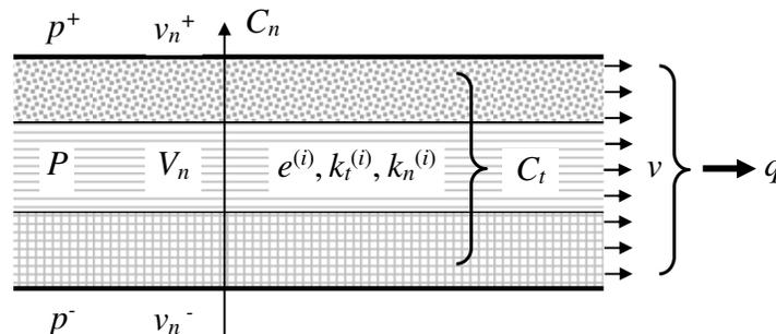
Concerning the flow perpendicular to the fracture, we note that  $v_n^+$  and  $v_n^-$  are the flow *in the matrix* perpendicular to the fracture and  $V_n = (v_n^+ + v_n^-)/2$ .
