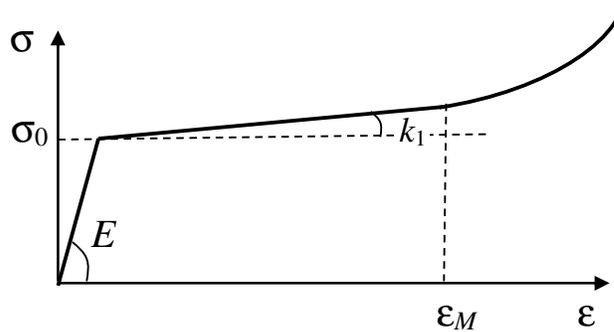
The curve presents, after the elastic limit, a long plastic stage with zero to small slope followed by a quickly increasing slope.
