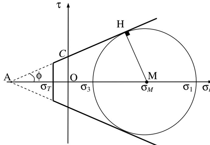
Flow rule:  $\dot{\boldsymbol{\varepsilon}}^p = \dot{\lambda} \frac{\partial G}{\partial \boldsymbol{\sigma}}$  or more precisely  $\dot{\boldsymbol{\varepsilon}}^p \in \frac{\partial G}{\partial \boldsymbol{\sigma}}$  (external normals cone for singular points, with:
