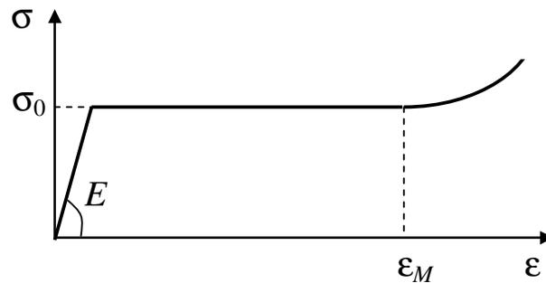
Under a uniaxial stress, the deformation is elastic and linear up to the stress  $\sigma_0$  for the axial strain  $\epsilon_0 = \sigma_0/E$  and then a perfect plastic strain takes place up to a total axial strain  $\epsilon_M$ . After this stage, the stress increases with a curve which is a quadratic function of the plastic strain.
