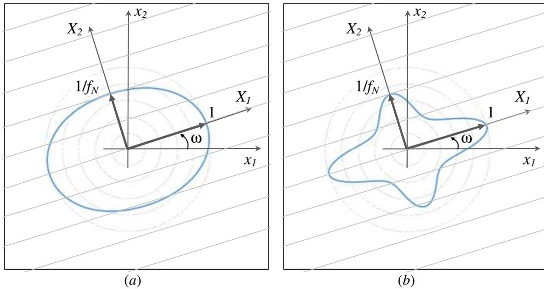
Figure: Different cases of UCS anisotropy: (a) Weak anisotropy for rock matrix:  $\omega=18^\circ$ ,  $a_T^p = 0.4$ ,  $b_T^p = 0$  and (b) anisotropic UCS for a jointed rock:  $\omega=18^\circ$ ,  $a_T^p = 0.4$ ,  $b_T^p = 1.5$
