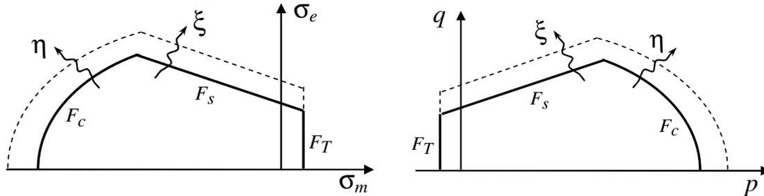
Figure:  $F_s$  : Shear criterion (Mohr-Coulomb),  $F_T$  : Traction cutoff,  $F_c$  : Compressibility
