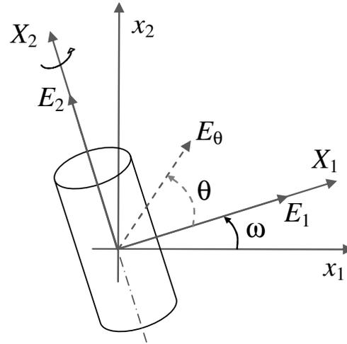
The model can include a rotation  $\omega$  of  $X_2$  with respect to the  $x_2$ -axis in the plane of calculation ( $x_1, x_2$ ). Note that the out-of-plane modulus  $E_3$  will be equal to  $E_1$ .
