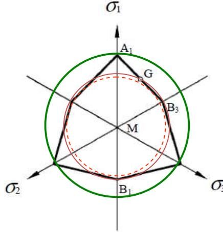
Equivalent Drucker-Prager parameters for Mohr-Coulomb: Option 1: circle passing by external corners (green circle), Option 2: passing by internal corners (red circle), Option 3: tangent to faces (dashed-line circle).
