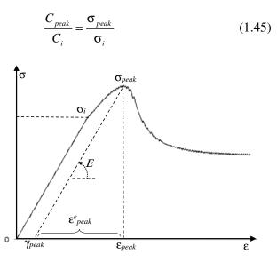
**Figure**: Determination of  $\gamma_{peak}$  and  $\sigma_{peak}$  from experimental curves
