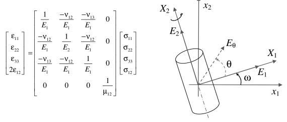
The model can include a rotation  $\omega$  of  $X_2$  with respect to the  $x_2$ -axis in the plane of calculation  $(x_1, x_2)$ . Note that the out-of-plane modulus  $E_3$  will be equal to  $E_1$ .
