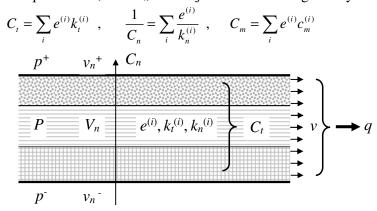
Concerning the flow perpendicular to the fracture, we note that  $v_n^+$  and  $v_n^-$  are the flow *in the matrix* perpendicular to the fracture and  $V_n = (v_n^+ + v_n^-)/2$ .
