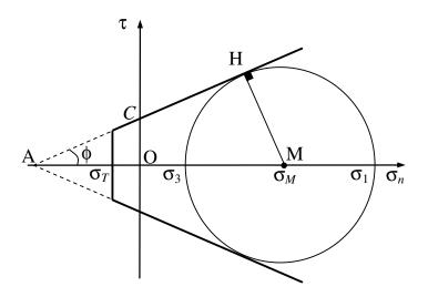
Flow rule:  $\dot{\mathbf{\epsilon}}^{p} = \dot{\lambda} \frac{\partial G}{\partial \mathbf{\sigma}}$  or more precisely  $\dot{\mathbf{\epsilon}}^{p} \in \frac{\partial G}{\partial \mathbf{\sigma}}$  (external normals cone for singular points, with:
