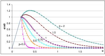
Traction-Separation curves for different  $\beta$  values
