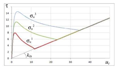
Shear stress versus slip under different compressive normal stresses for the option without plasticity: the curves join and follow the elastic line with residual stiffness  $k_{0t}$
