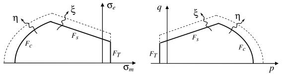
Figure:  $F_s$ : Shear criterion (Mohr-Coulomb),  $F_T$ : Traction cutoff,  $F_c$ : Compressibility  $(q = \sigma_e, p = -\sigma_m)$
