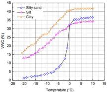
$W_c$ : unfrozen water content of the partially frozen soil  $W_c^{Max}$ : water content of the unfrozen soil
