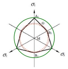
Equivalent Drucker-Prager parameters for Mohr-Coulomb: Option 1: circle passing by external corners (green circle), Option 2: passing by internal corners (red circle), Option 3: tangent to faces (dashed-line circle).
