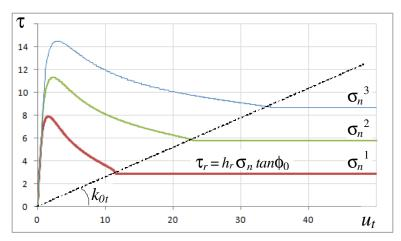
Shear stress versus slip under different compressive normal stresses for the option with plasticity
