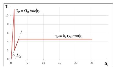
Shear stress versus slip for the option with plasticity and brittle damage ( $\beta < 1$ )
