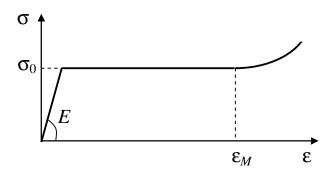
Under a uniaxial stress, the deformation is elastic and linear up to the stress  $\sigma_0$  for the axial strain  $\varepsilon_0 = \sigma_0/E$  and then a perfect plastic strain takes place up to a total axial strain  $\varepsilon_M$ . After this stage, the stress increases with a paste which is a quadratic function of the plastic strain.
